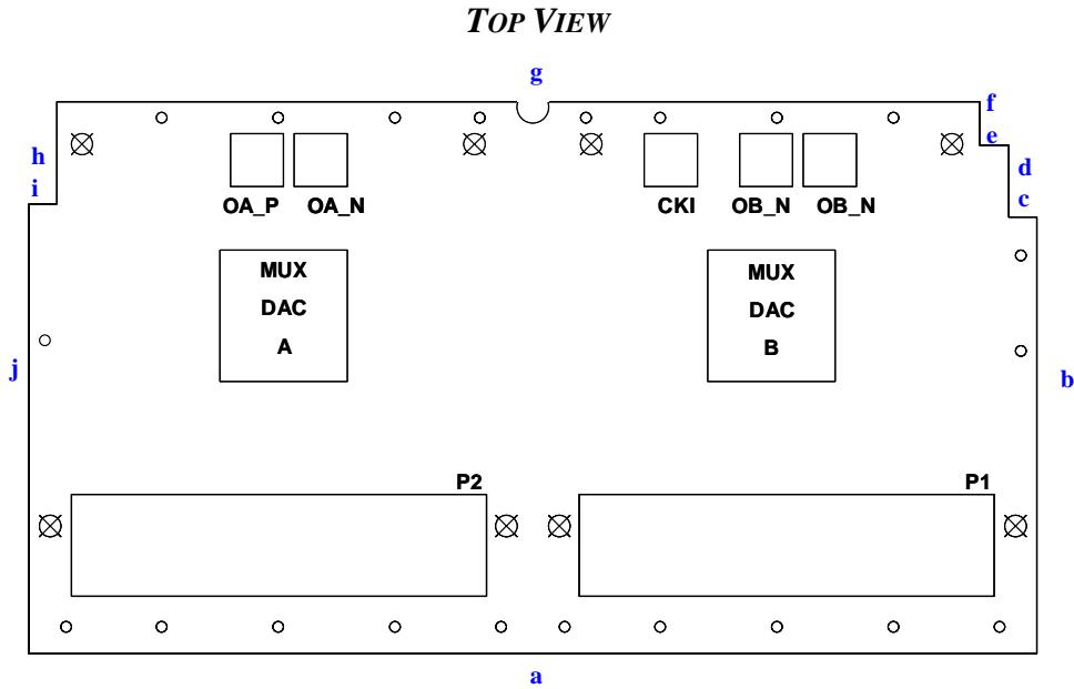
P1 is the primary HPC connector and P2 is the LPC connector. All dimensions use the bottom left corner of the board as the origin. All dimensions are in millimeters (mm). Board thickness is 1.62 mm.
